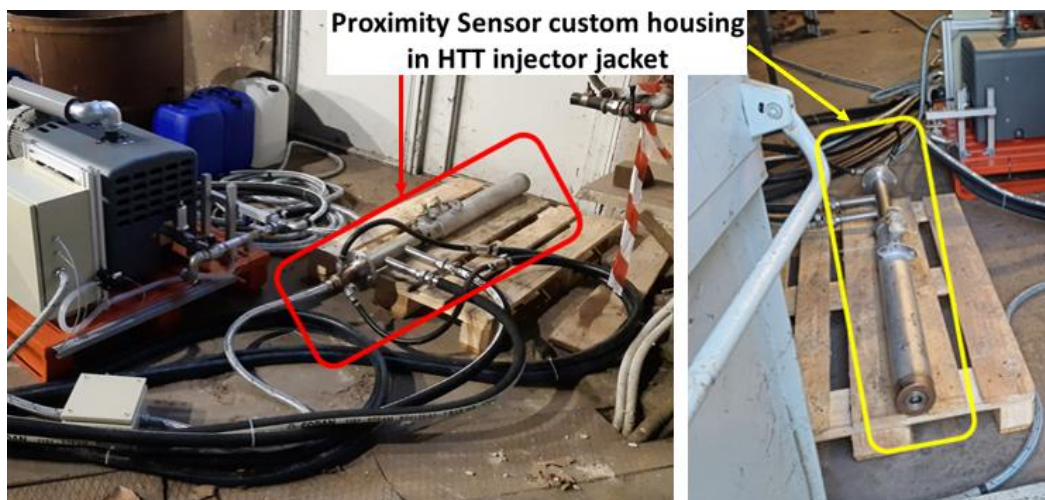
Figure 26 - Proximity Sensor custom housing lance during preliminary tests at the RINA CSM facilities in Rome
