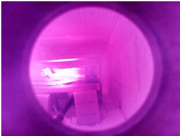
Figure 44 - View of the interior of the furnace when the thermocouples measured 900°C
