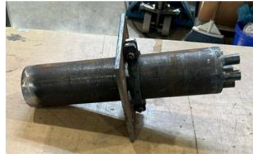
Figure 31 - Water-cooled flange for semi-industrial test at Dalmine reheating furnace
