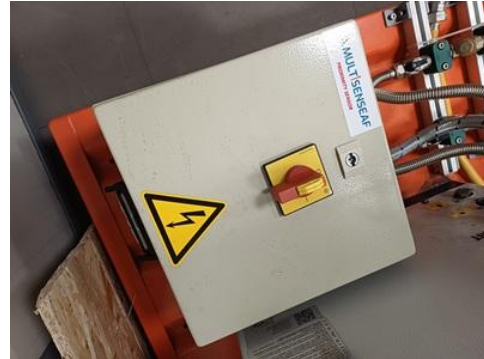
Figure 11. Water-cooling chiller electrical box
