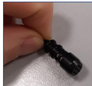
Microphone with 8mm diameter
