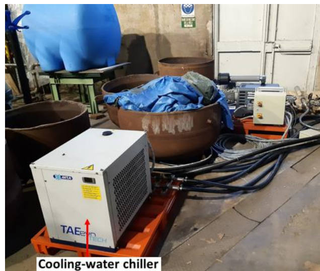
Figure 27 - Proximity Sensor cooling water chiller during preliminary tests at the RINA CSM facilities in Rome
