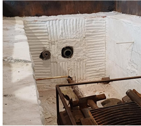
Figure 39 - Proximity sensor flush with inner furnace surface
