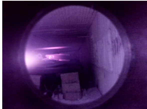
Figure 43 – View of the interior of the furnace when the thermocouples measured 600°C
