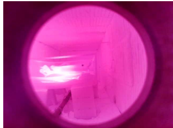
Figure 45 - View of the interior of the furnace when the thermocouples measured 1160°C
