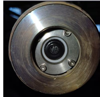
Figure 59 - Lance tip without protective glass
