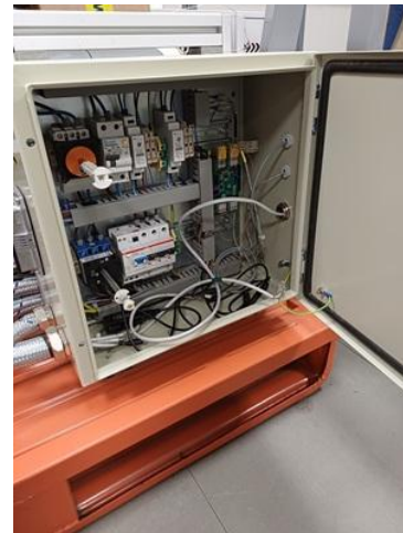
Figure 12. Blower electric box that manages the three-phase power supply for the air pump's on/off control
