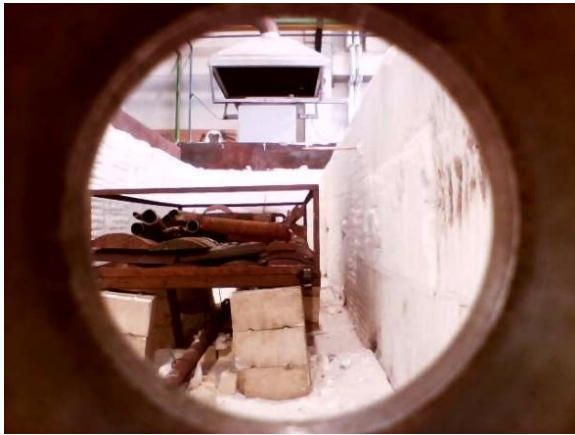
Figure 42 - Scrap basket inside the furnace when it was still open
