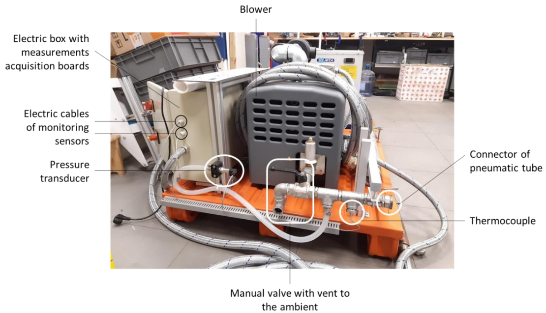
Figure 9. Pallet with compressed air blower and electric box
